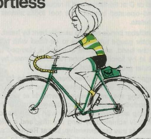
Modern road surfaces are generally good—but even so, if our front forks were rigid we would have a very uncomfortable ride, and use up so much energy absorbing the vibration in our arms that mileages would tumble and times would stretch alarmingly. So the front fork blades are curved to a carefully planned “rake” to provide resilience and so smooth out some of the road-roughness.
