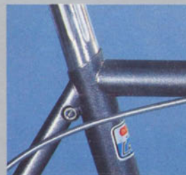
Brazed-on frame integrated seat post clamp
