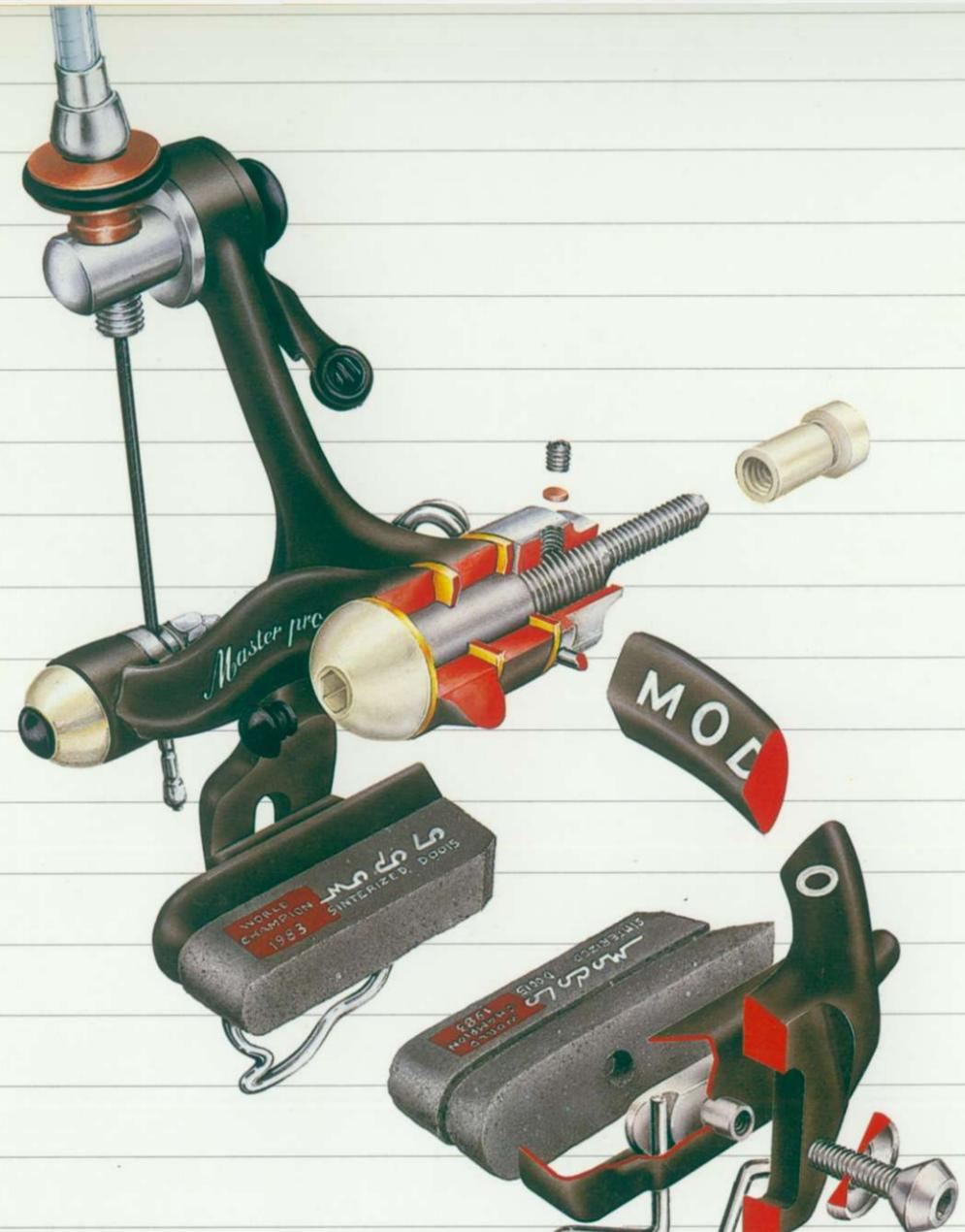
Exclusive cable blocking system which maintains the cable always in axial position (Intern. patent).
