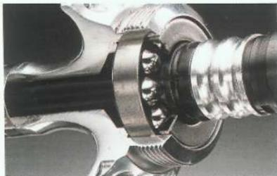
lease mechanism of this hub uses a hardened, tempered steel skewer and locknut and employs the classic eccentric closure design which remains the standard of the industry.
