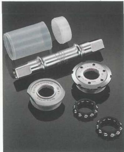
The bottom bracket is the same race-proven design that has won more races in professional competition than all others combined. It uses an axle and cups made of case-hardened steel. The rolling mechanisms are composed of hardened chromium steel balls with diameter 1/4" and held together in resin retainers.
