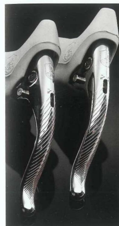
under any condition whether it be the cold, wet racing environment of Northern Europe or the dry sizzling heat of the California desert. The brake pad holders are uniquely designed so that they can be adjusted for correct toe-in and to compensate for any rim shape in order to provide 100% surface contact. The brake shoes themselves can be raised or lowered on the caliper arms as usual.
