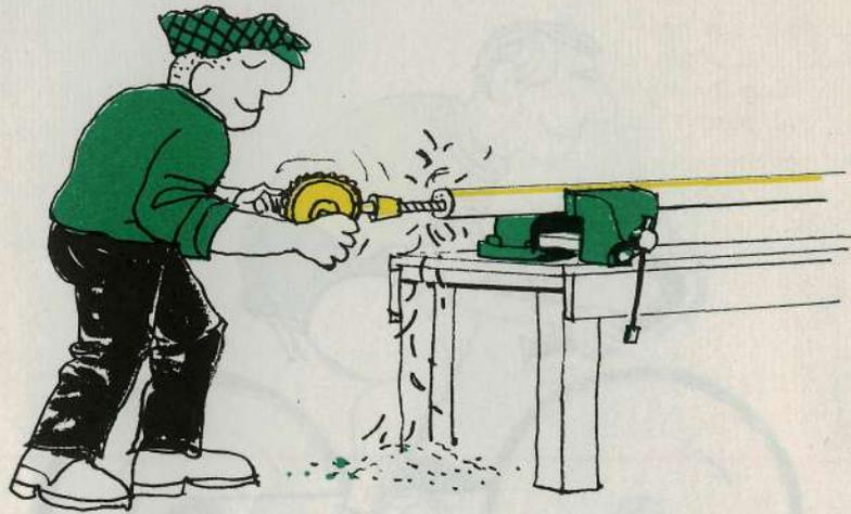
Anyone thinking for the first time about tubing is immediately interested to know how the hole got there. Was an accurate hole taken and wrapped up in steel, or was a very strong hole pushed firmly through a steel bar? Actually, both ways are used, for different applications. For some of the "lower orders" of the cycling world (junior cycles, tradesmen's bikes, roadsters), a strip of steel is, in fact, wrapped by a series of shaped rollers "round a hole" and the seam electrically welded.
