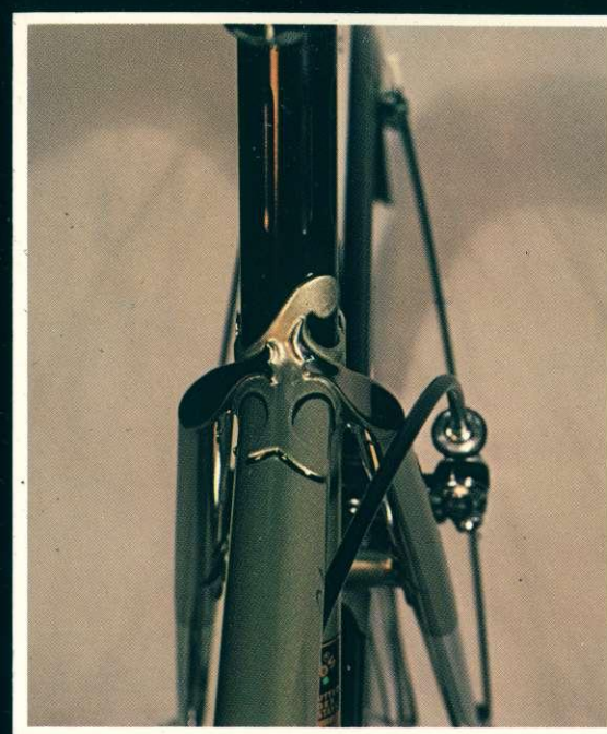
Custom cut seat lug and semi-wrap seat stays
