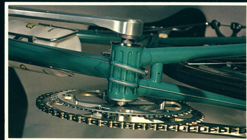
Nylon lined cable guides under a relieved bottom bracket
