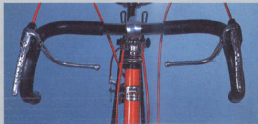
WEINMANN side pull with AUTO-LUBE cables
