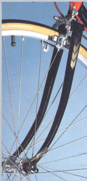
Sloping crown fork and quick release
