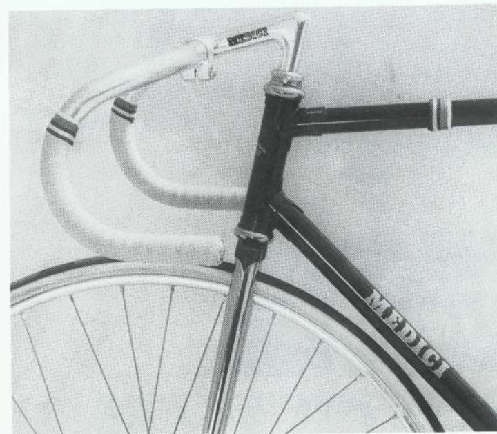
No room for error!! Note sharp, crisp lug & crown work.
